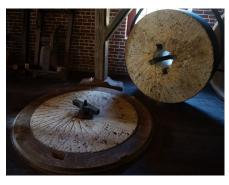
wheat berries into fine flour. While this technology has been known for many centuries, it is still an awe inspiring adventure to watch it in operation at the mill. The moving or runner stone on top must be perfectly balanced on a dime sized steel spindle protruding through the base stone. It must be perfectly balanced and level so that it maintains a paper thin separation from the base stone without ever touching it while spinning at some 80—90 revolutions per minute for hours at a time.
